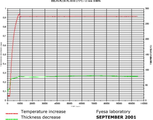
**CREEP DEFORMATION / HOT CREEP TEST**
