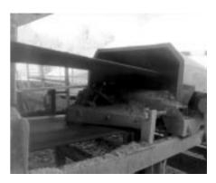
The cleaner PLG is for belt widths of 400, 500 and 650 mm. To be installed near to the drive drum.
